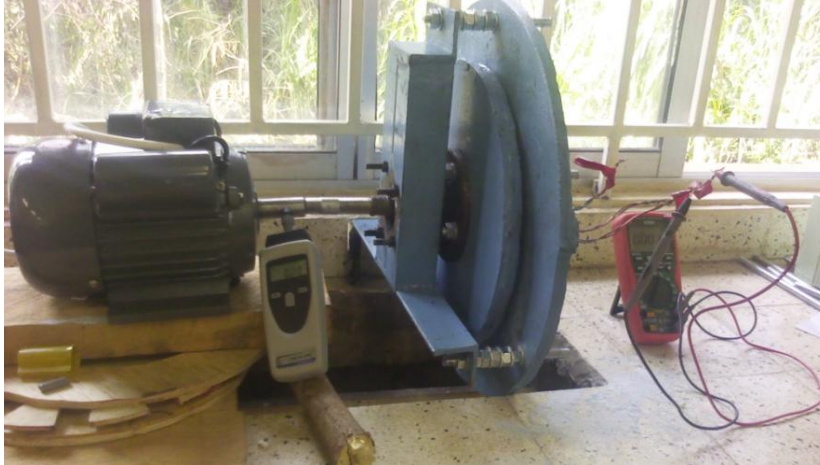
Figure 7: Generator test-set up
