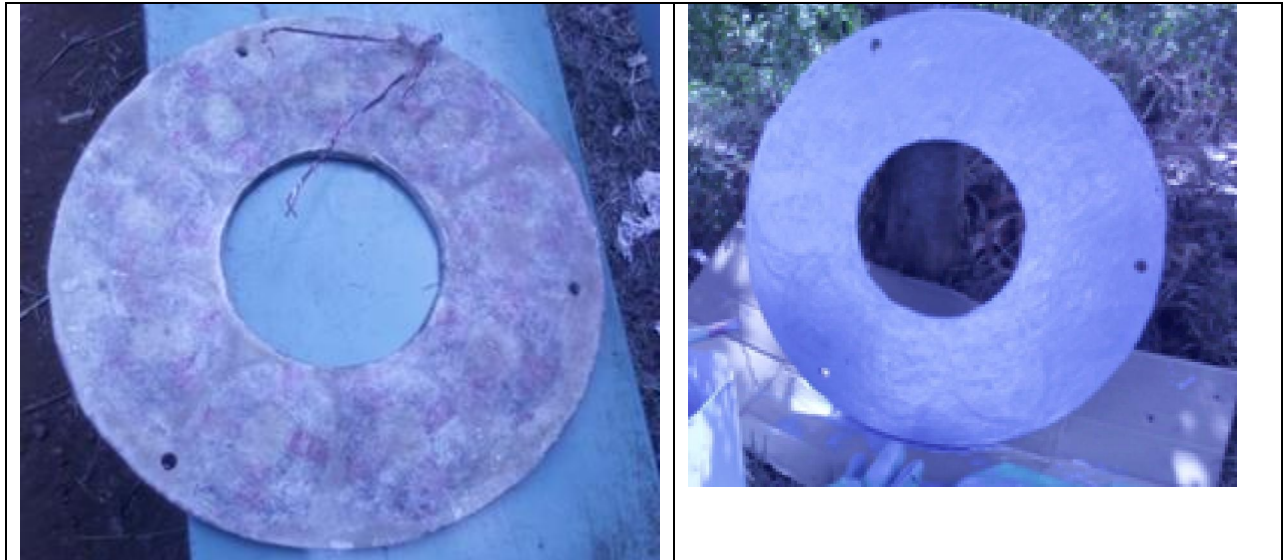
Figure 4: Complete stator before and after painting
