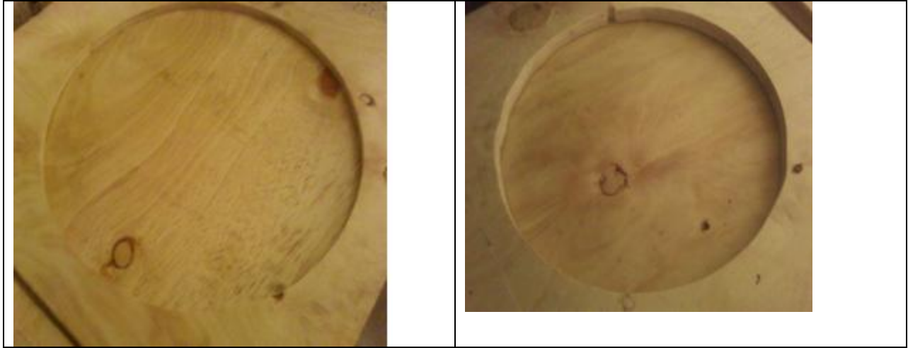
Figure 2: Finished stator and rotor moulds
