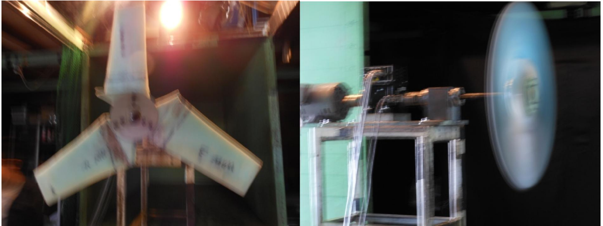
Figure 7: Wind tunnel testing of the turbine rotor
