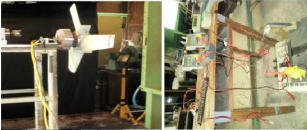
Figure 9: Testing the wind electric generator for electricity production
