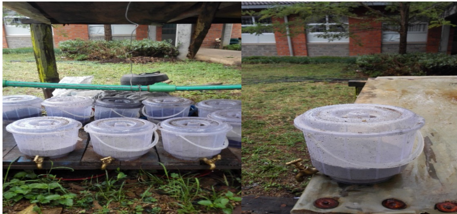
Figure 0.5: 2kg containers with the crushed adsorbents
