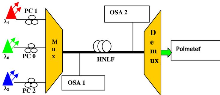
Figure 1: set up. Polmeter: Polarimeter
