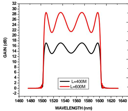
Figure 6(a): graph of gain against wavelength, nonlinear coefficient,  $\gamma = 10$  sW<sup>-1</sup>
