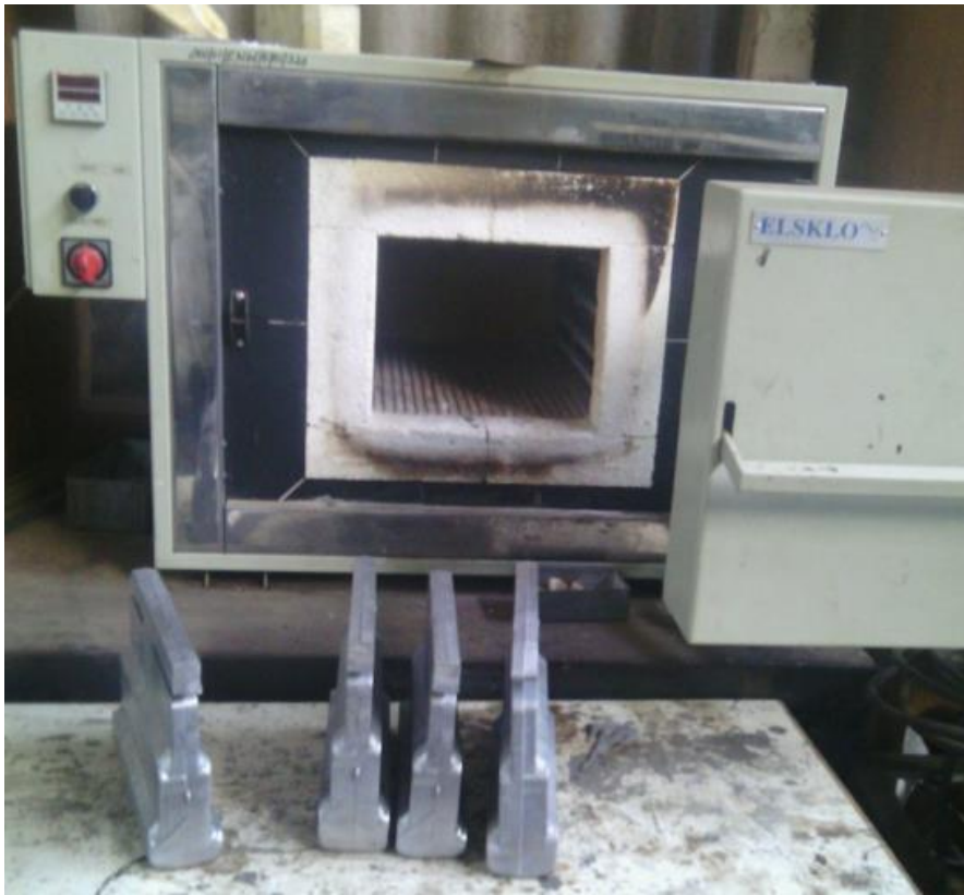
Figure 3.4: A photograph of the air circulated electric resistance furnace used for heat treatment.
