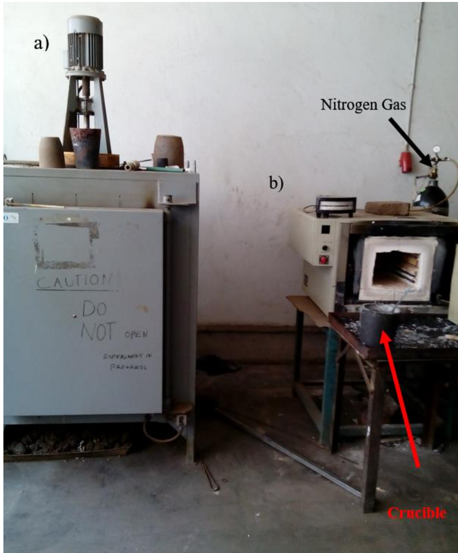
Figure 3.1: a) Air circulated furnace and b) Electric muffle furnace
