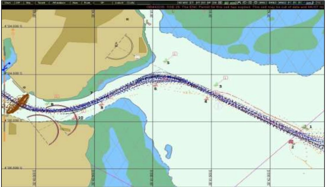
Figure 4.4 Channel orientation and Visual AtoN arrangement as shown by AIS track on Mombasa approach channel
