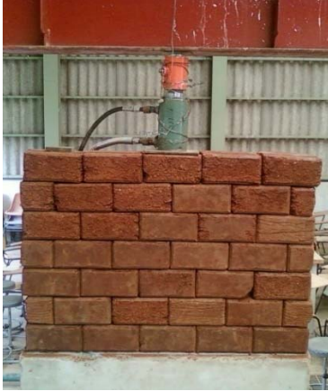
Figure 1: Typical arrangement of wall model for testing
