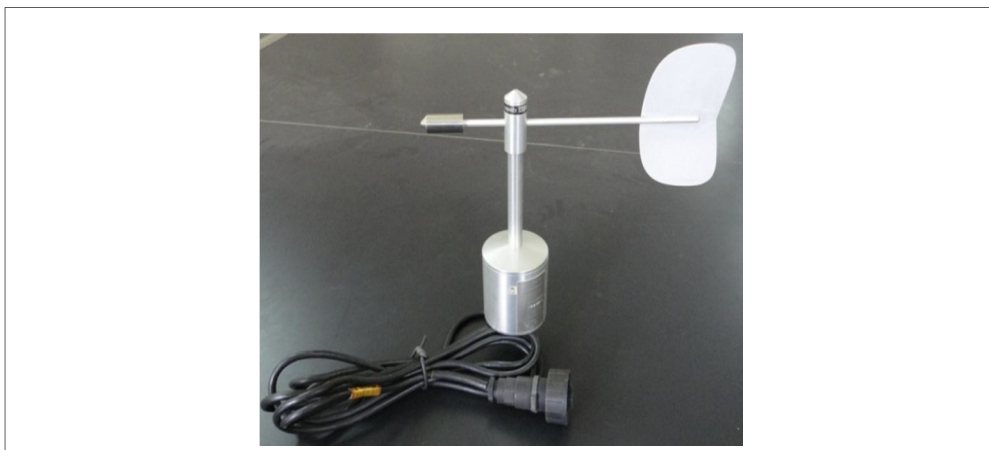
Plate 2: The wind vane sensor connected with weighted pointer
