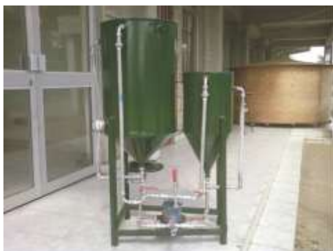
Figure 1: The fabricated biodiesel processor used during the study of animal fat biodiesel production and evaluating its potential as an alternative fuel.
