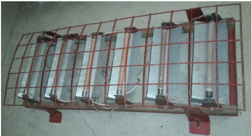
Figure 2.7: Space heater for a 3-phase load
