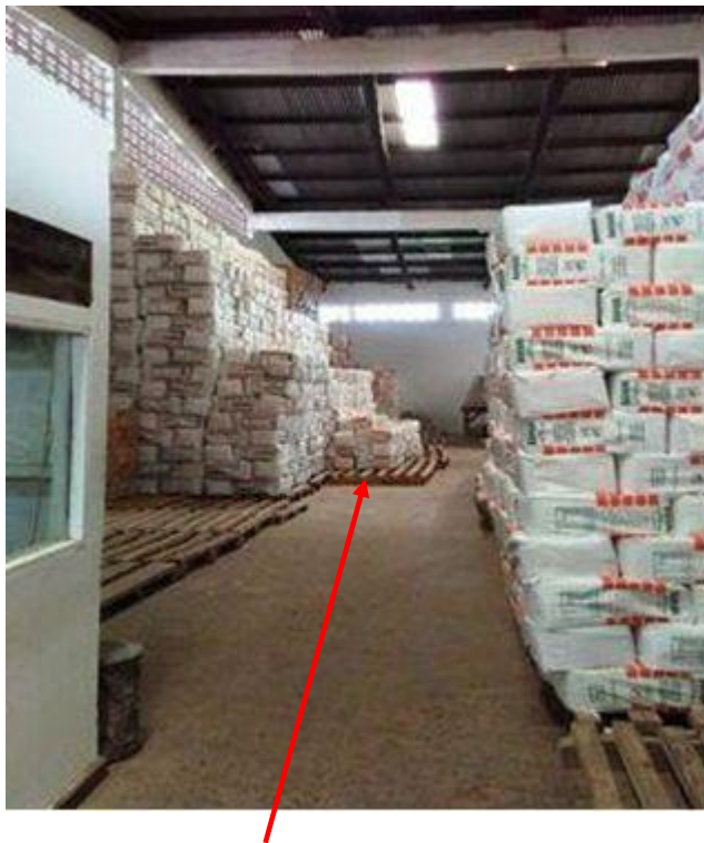
Plate 4.7: High unsafe stacking and obstructed gangway
