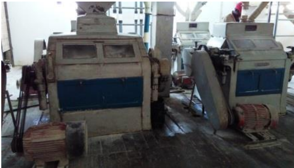
Plate 4.1: Unguarded milling machines
