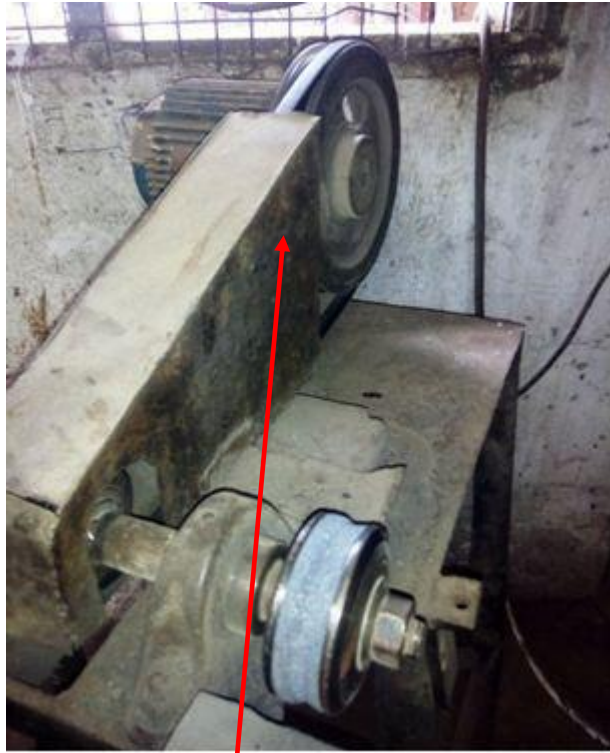
Plate 4.6: Partially guarded machine in the workshop
