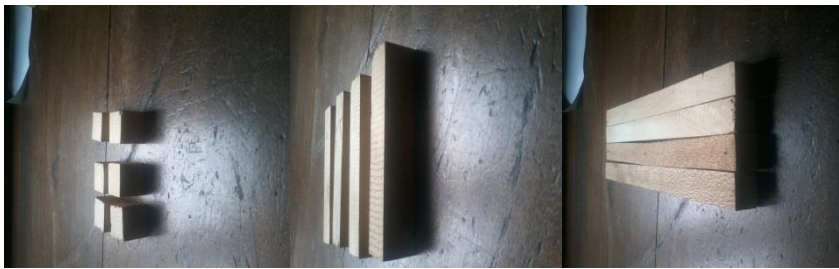
Plate 3.18: Pictorial views of samples used for testing shear strength, compressive strength and janka hardness.
