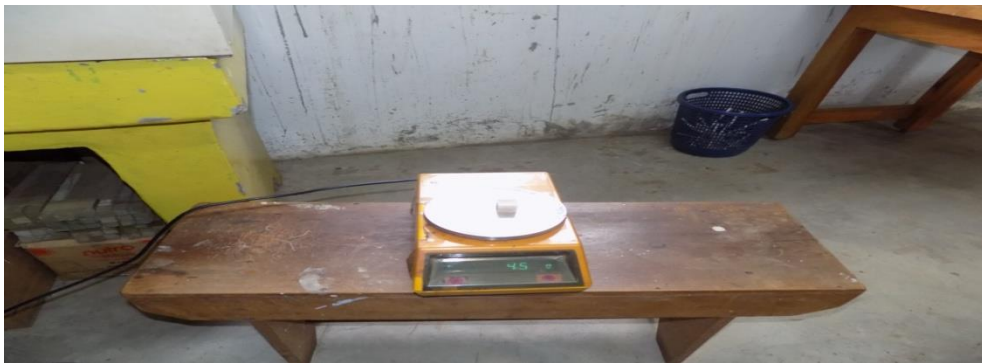
Plate 3.4: A view of a weighing scale used to measure weight of specimens in grammes.
