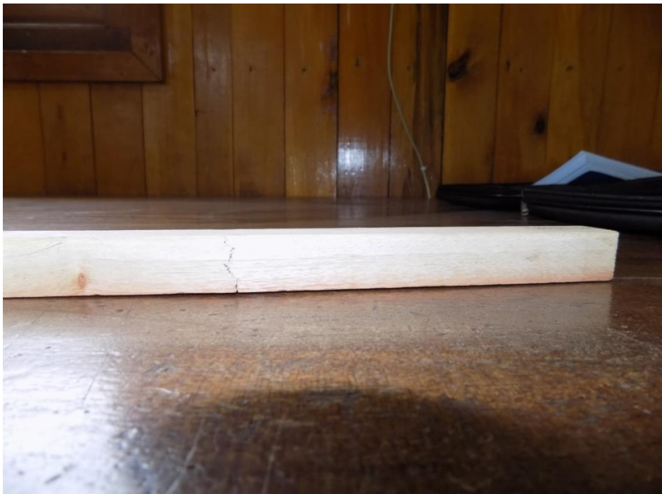
Plate 3.17: View of the specimen after the test showing the failure mode.
