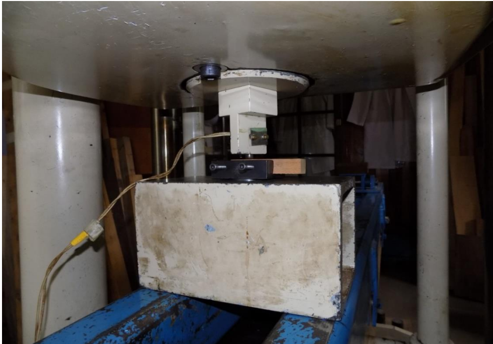
Plate 3.9: View of janka indentation tool and the specimen holder fitted on the moving cross-head of the universal testing machine.
