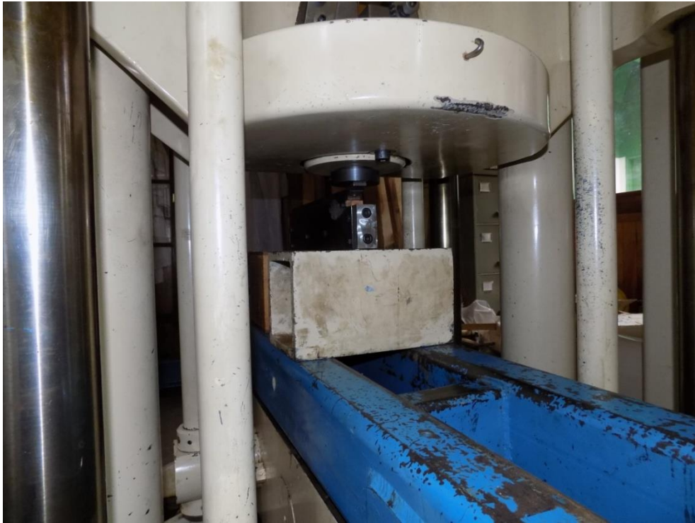
Plate 3.6: View of the compression plate and the shearing tool attached to the underside of the machine.
