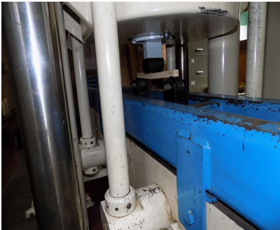
Plate 3.15: View of the Bending Knee and Trunion Supports attached at underside of moving cross- head of machine.
