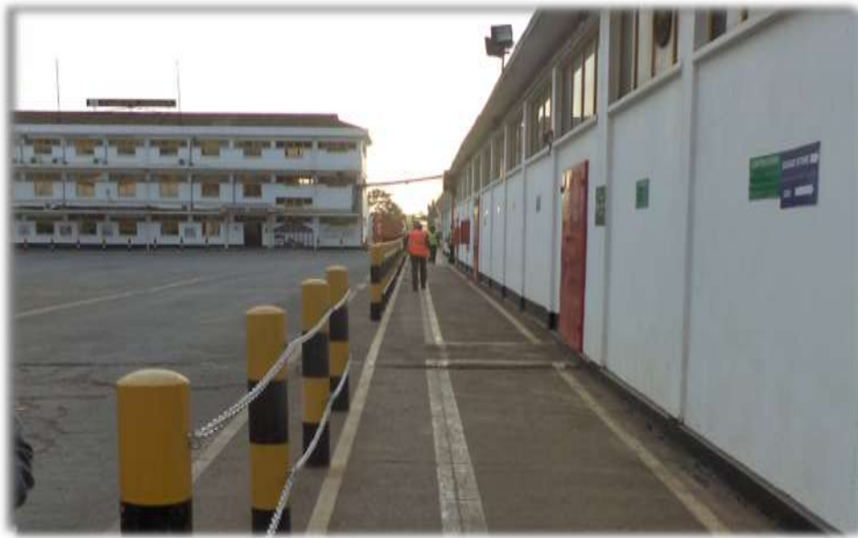
Plate 4.1: A safe walkway with clear segregation from vehicular traffic
