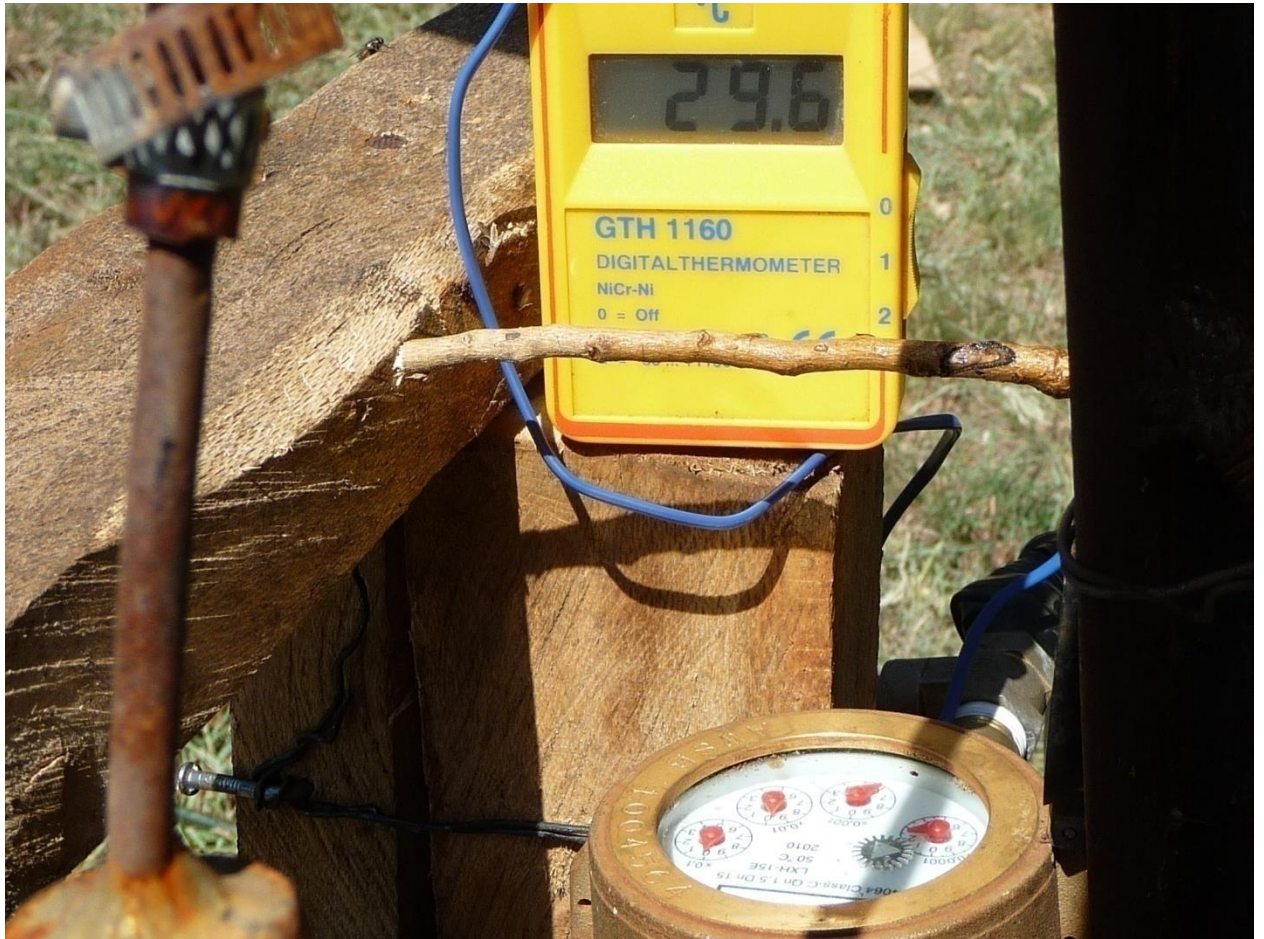
Plate A3: Flow Rate meter and thermocouple thermometer used in the experiments
