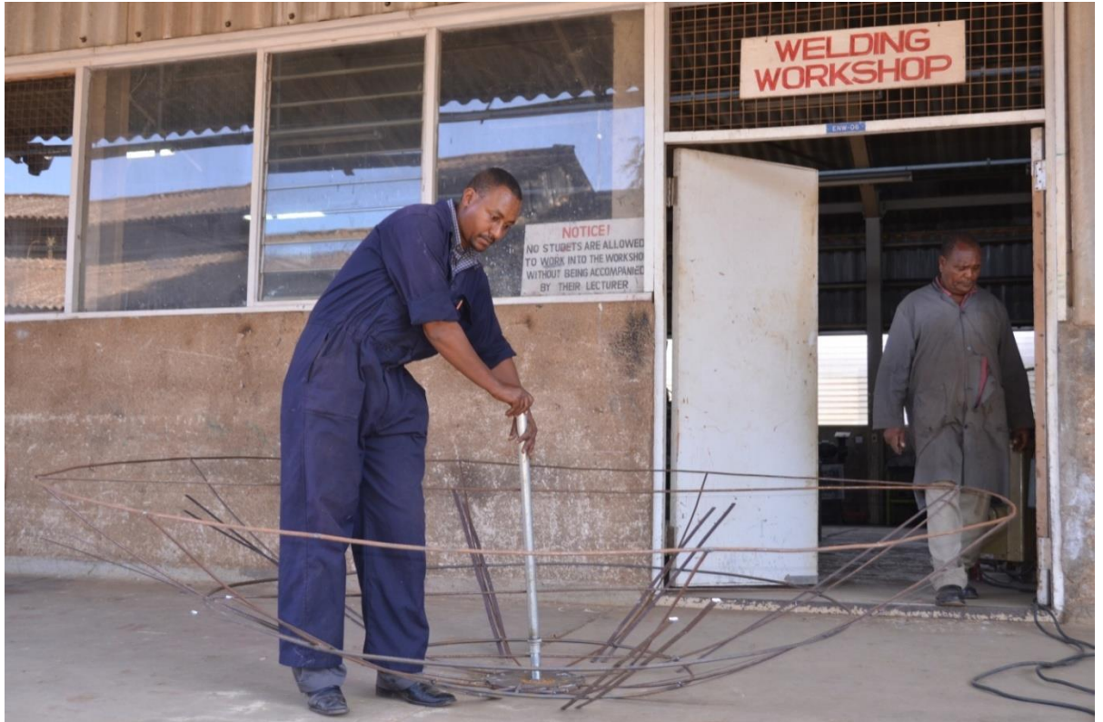
Plate A5: Construction of parabolic dish at engineering workshop JKUAT.
