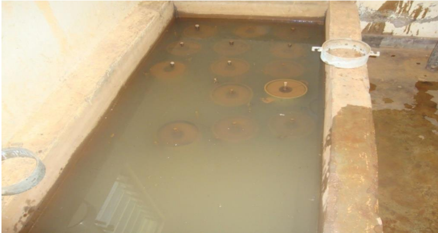
Plate 3-7: Soaked moulds for CBR
