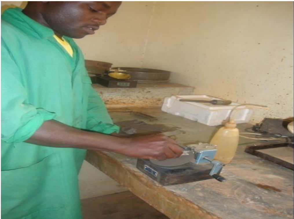
Plate 3-6: Dividing the sample by grooving tool on the Casagrande plate
