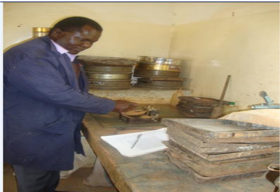
Plate 3.5 Author is setting up sieve analysis apparatus
