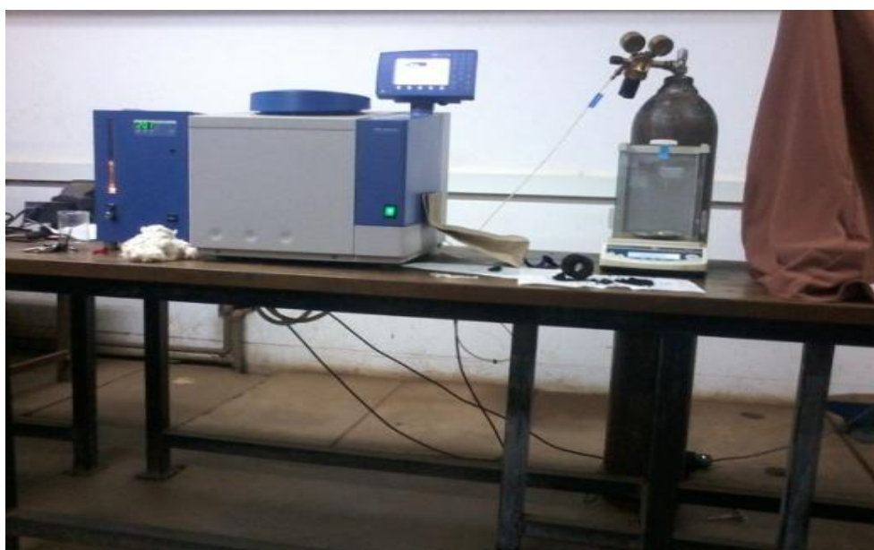
Figure 3.4: IKA KV600 digital bomb calorimeter (Staufen, Germany)
