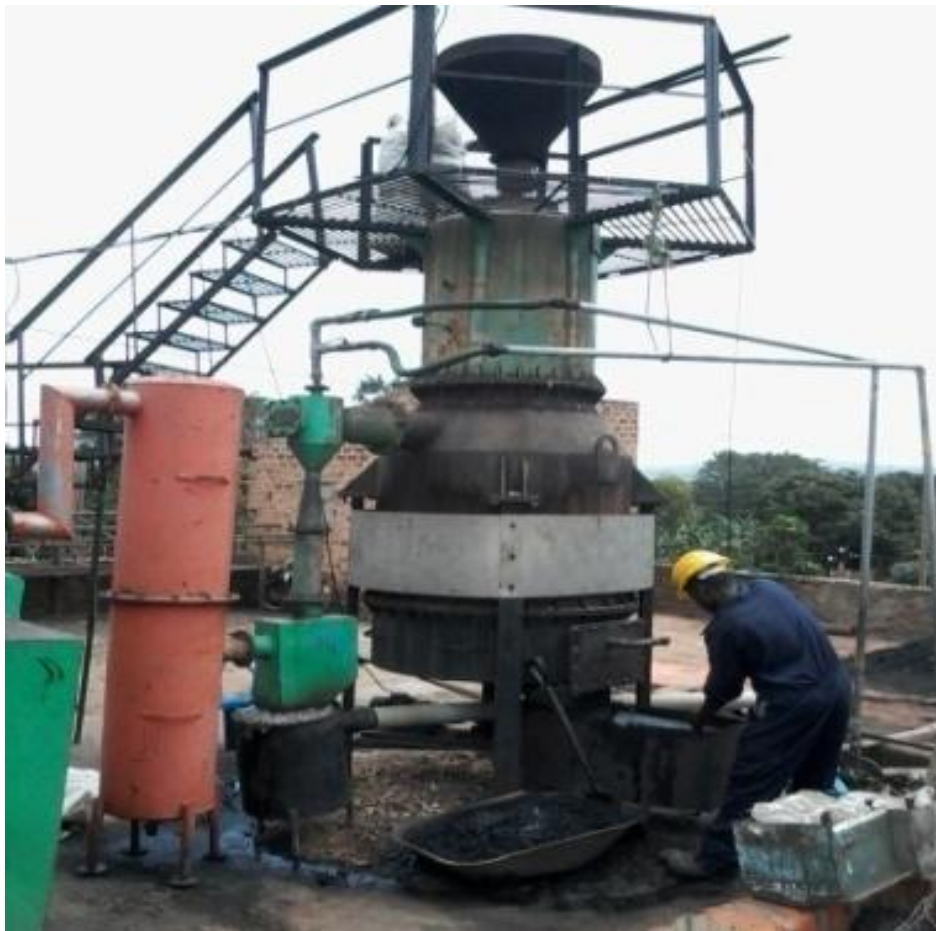
Figure 3.1: Gasifier used to carbonize maize cobs
