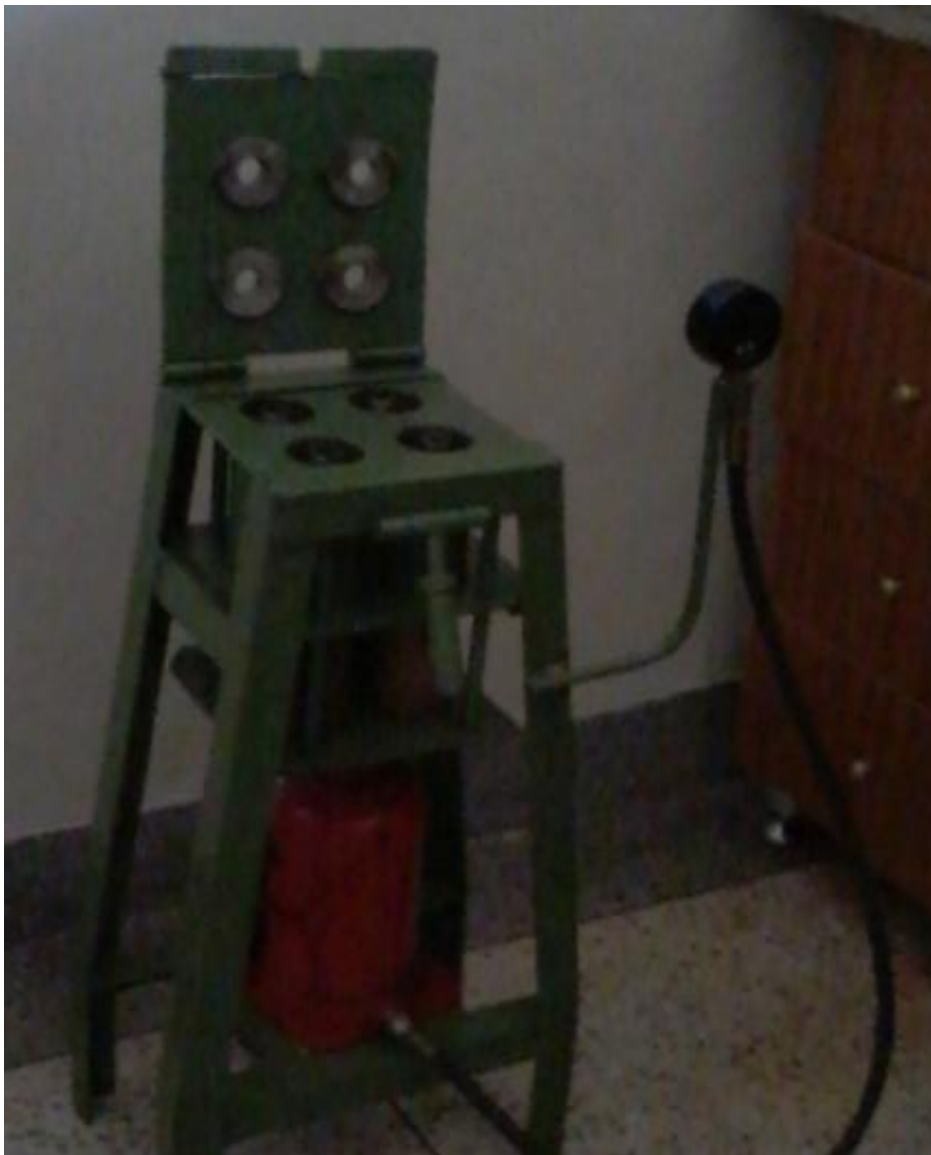
Figure 3.2: Hydraulic briquette press connected to pressure gauge
