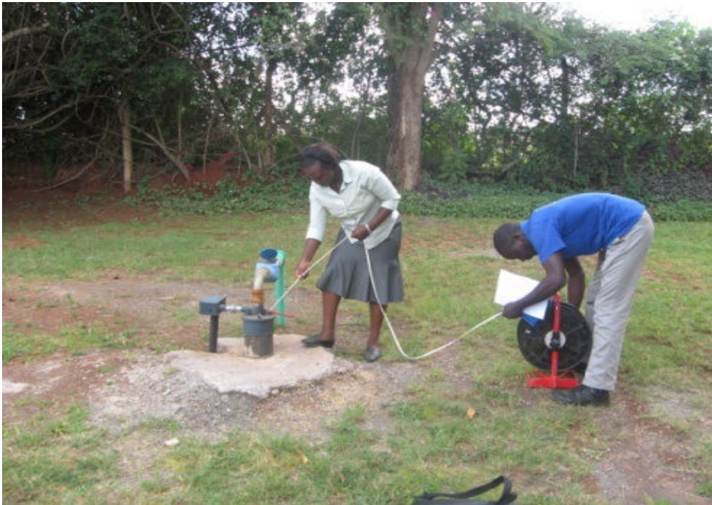
Figure 3.2: Measurement of groundwater levels
