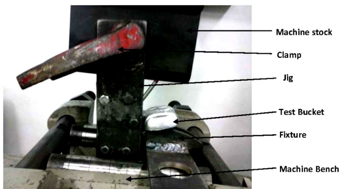
Fig. 4. Set up of the bending experiment
