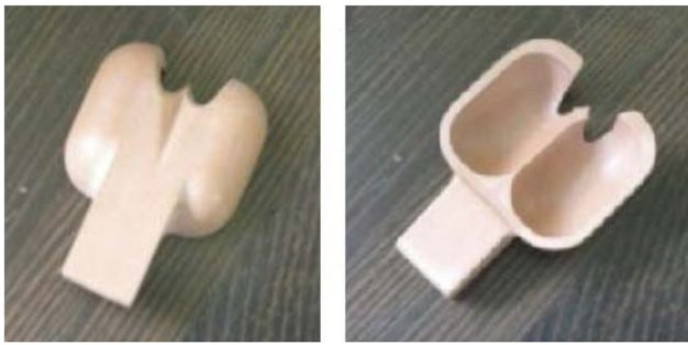
Fig. 3. Master pattern made from plastic
