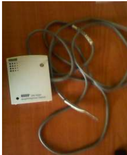
Figure 3.3 HOBO U12 Temperature/ Humidity/External Data Logger -U12-012
