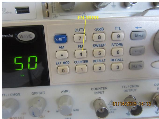
Figure 3.12: FM mode of the signal generator
