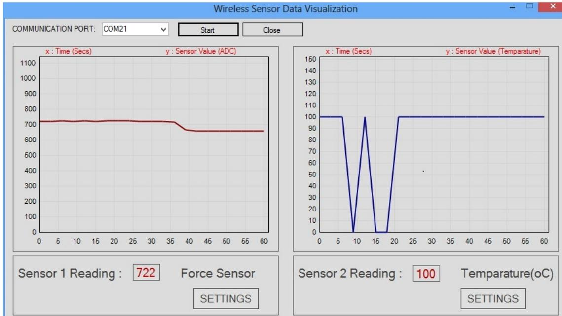
Figure 4.24: Snapshot of data received from WSN
