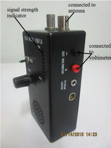
Figure 3.14: Field strength meter
