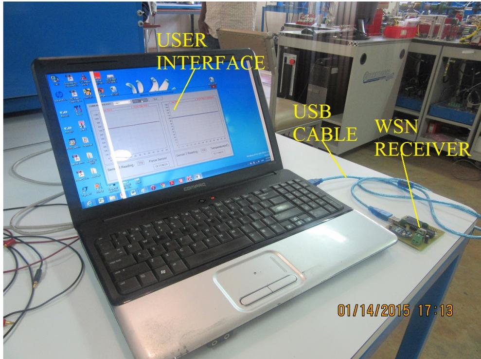
Figure 3.17: Receiver set-up
