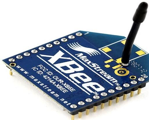
Figure 3.1: XBee Wireless Sensor Node [37]
