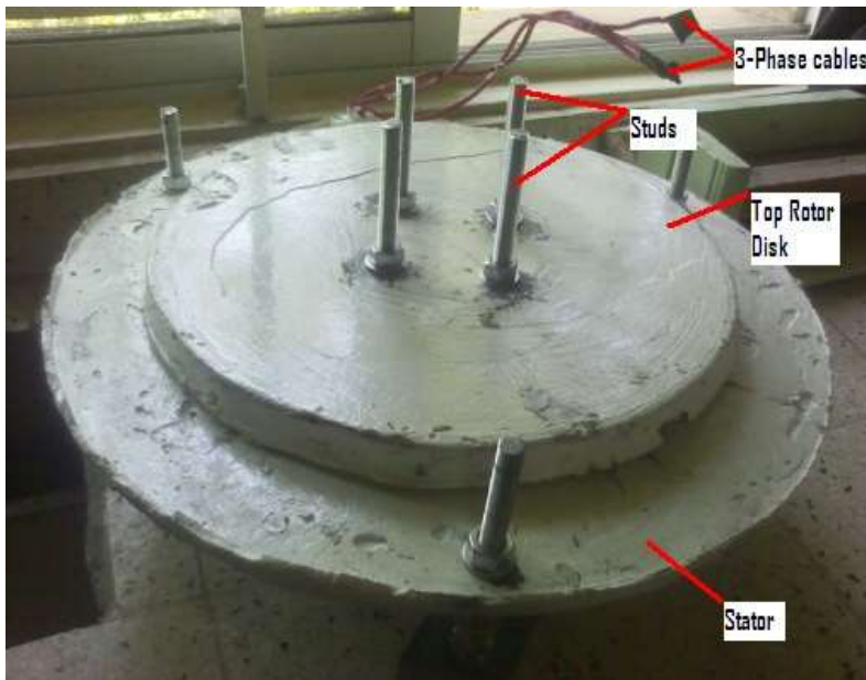
Plate 3.28: Assembled AFPM generator
