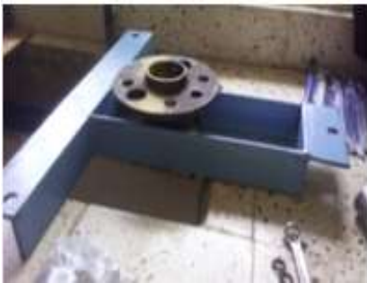
Plate 3.22: Car hub on frame
