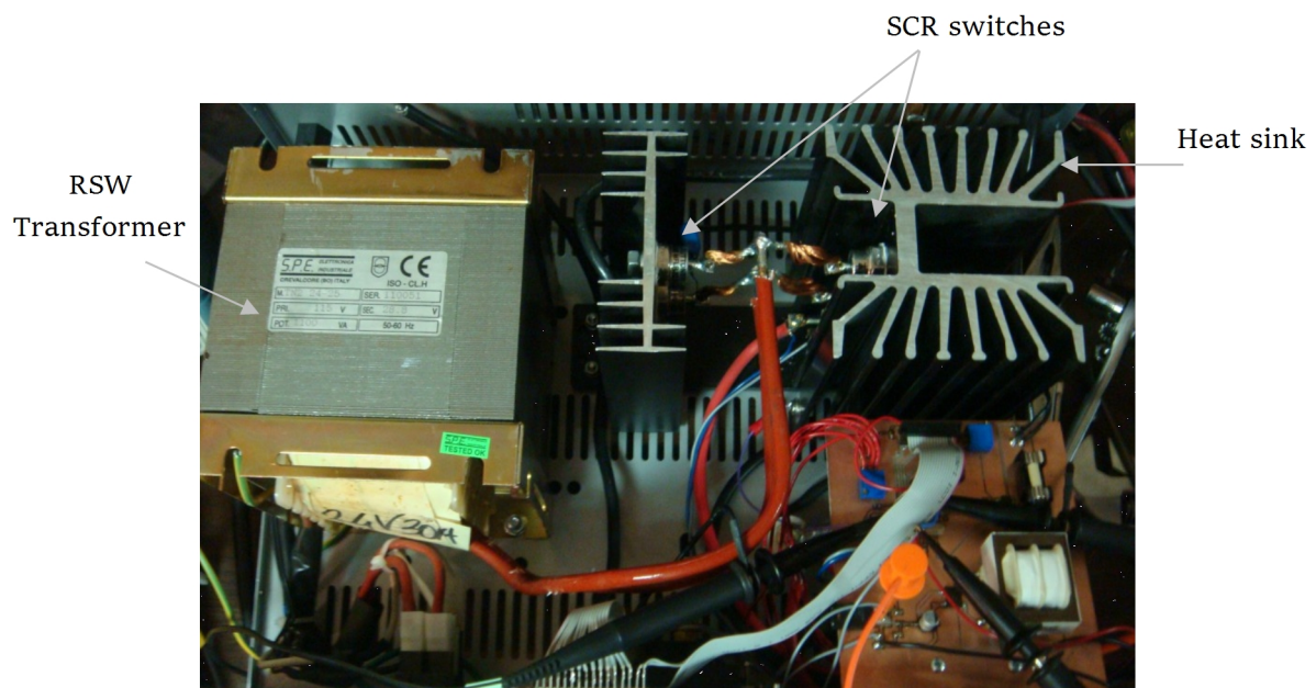
Figure 3.10: Experimental set-up for resistance spot welding.
