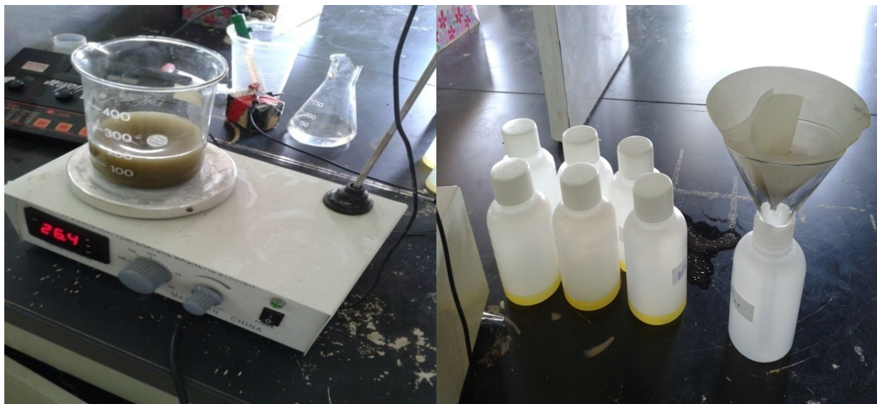
Figure 3-4: a) Sample stirring at speed of 150 rpm at room temperature and (b) filtration of the samples in the laboratory
