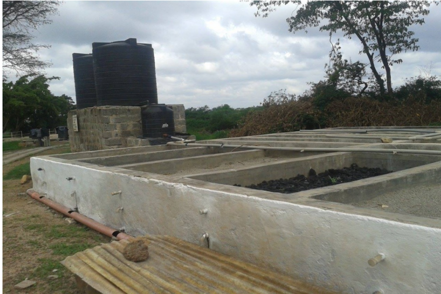
Figure 3-6: Set up of the constructed adsorbent bed system showing the elevated tanks, inlet and drainage pipes and the three sampling points along the depth of the adsorbent cells.
