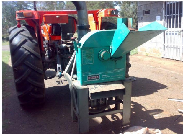
Plate 2.2: Disintegrator plant mill
