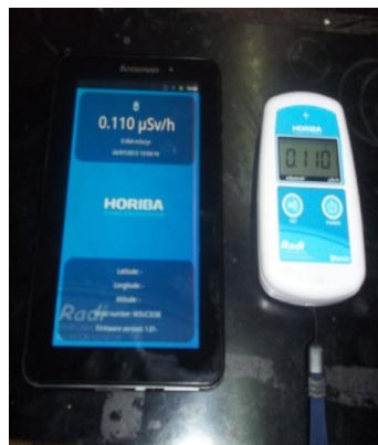
Plate 2.2: Bluetooth Connection of the radiation monitor to the GPS enabled Ipad.
