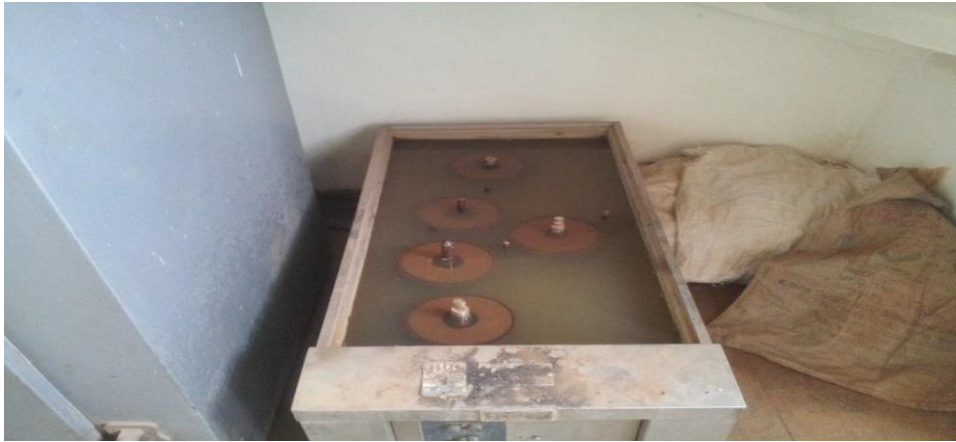
Fig. 8-15 Soaked samples for CBR Test
