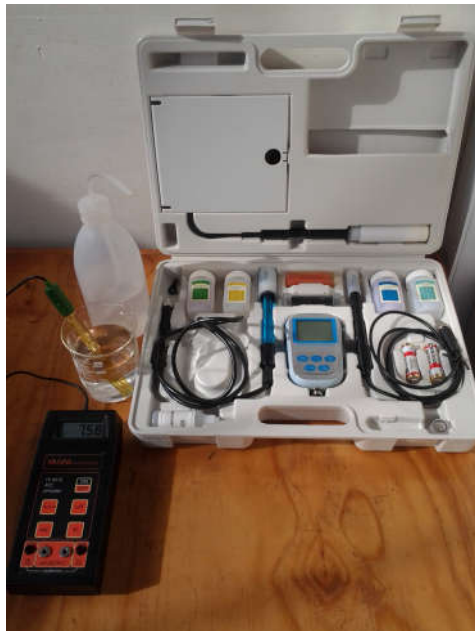
Figure 2.1: Plate of the Hanna pH meter (HI-8915) used in the experimental work
