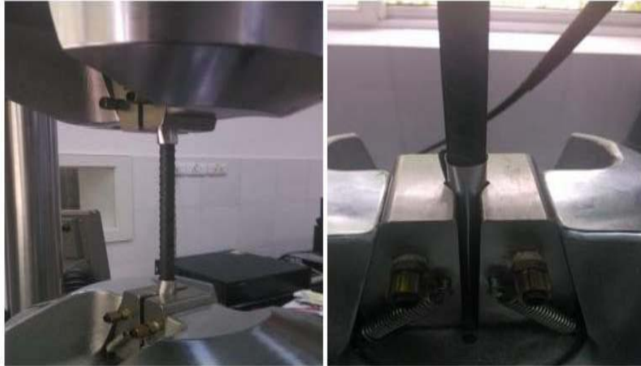
Plate 8: The servohydraulic testing machine with clamped test specimen
