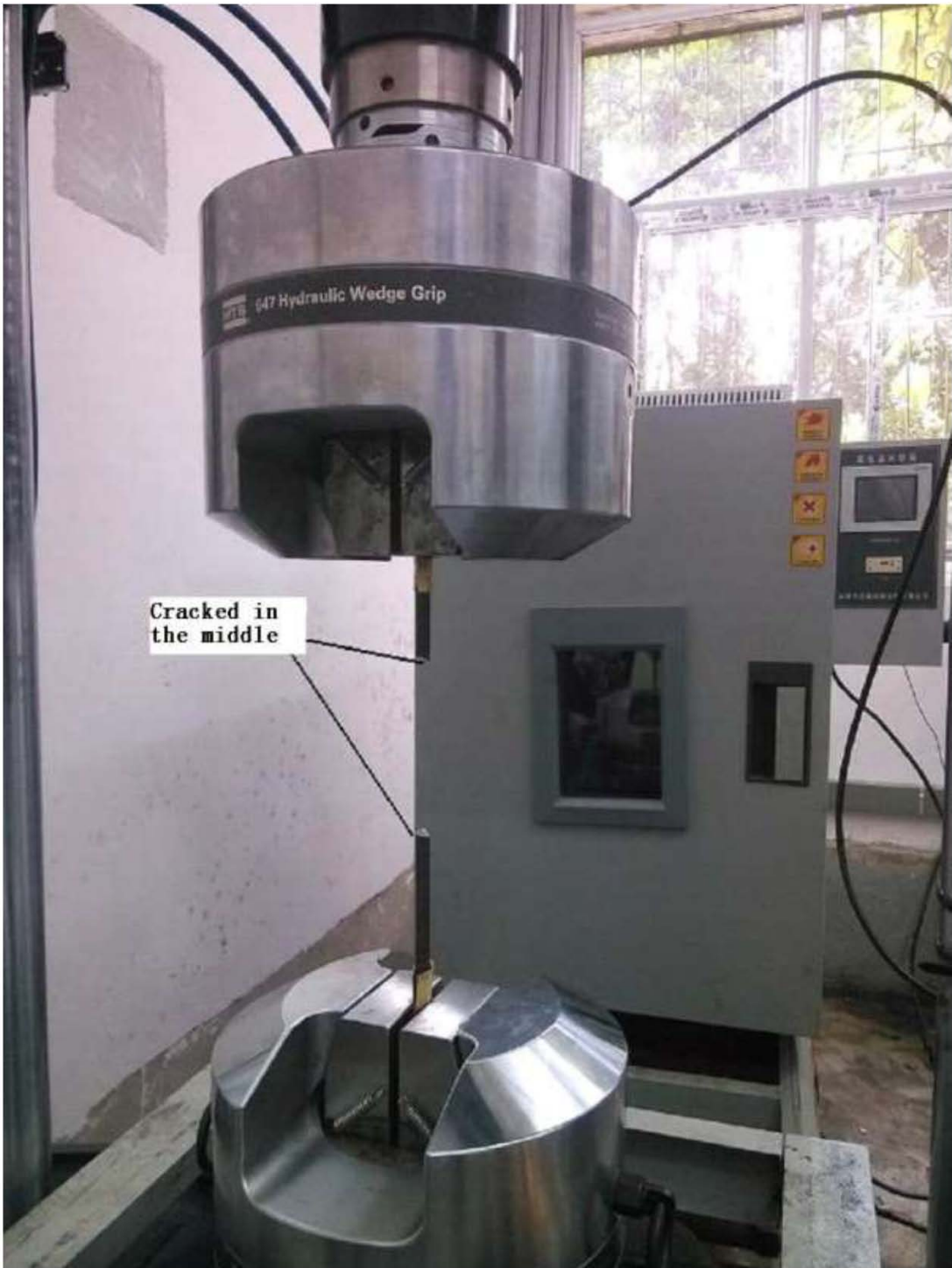
Plate 9: The MTS 810 fatigue machine with a specimen fractured at the centre
