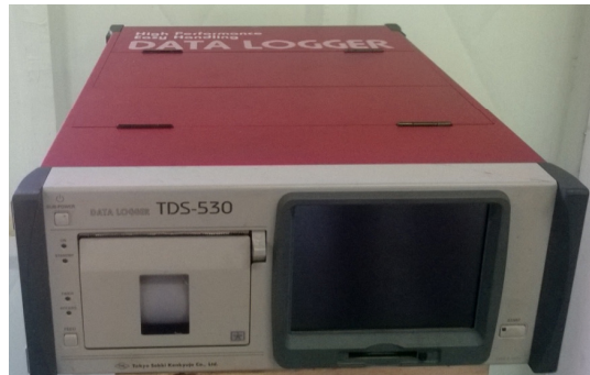
Figure 3.20: Multi-channel digital data logger
