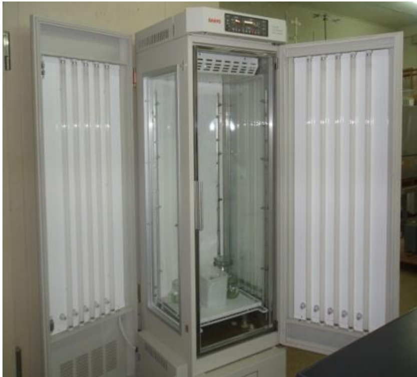
Figure 3.3 Showing the cool white fluorescent bulbs on all 4 sides to give uniform lighting in the growth chamber.
