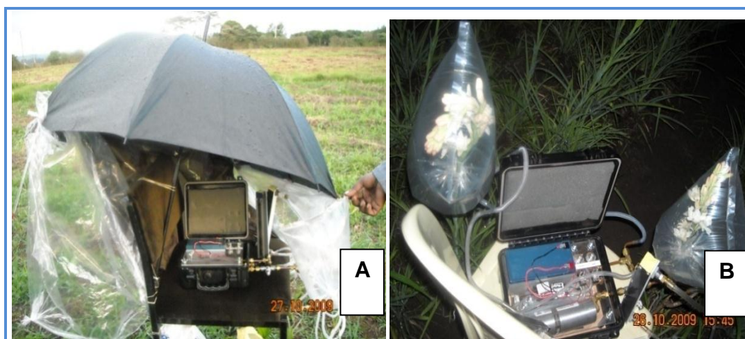
Figure 3.6 A) Makeshift tents for pump when there was drizzle in the field. B) The polyvinylacetate bag inflates and forms the chamber when air is pumped in
