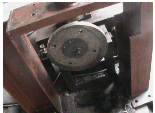
(b) Eccentric facility for adjusting crank 'radius'
