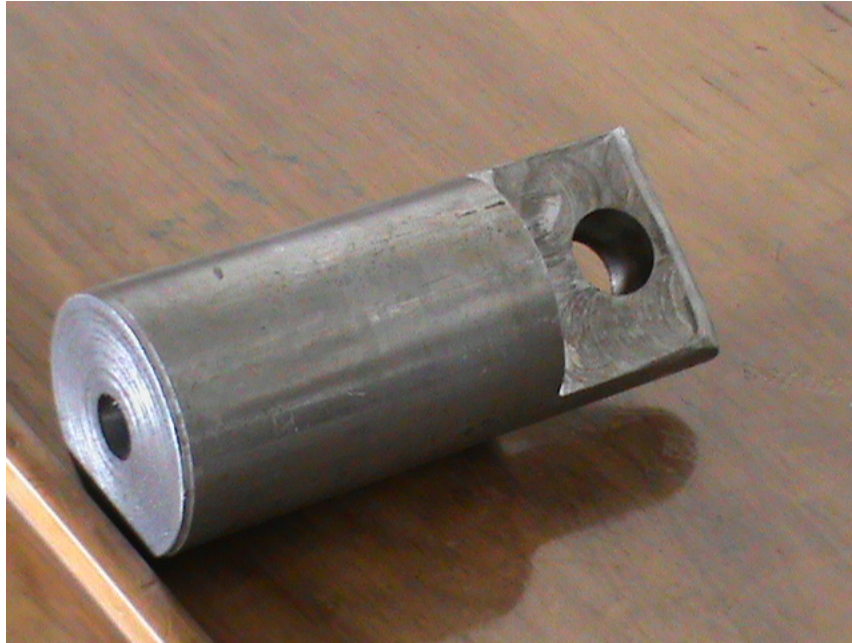
Figure 3.9: Gripper design for axial load fatigue test
