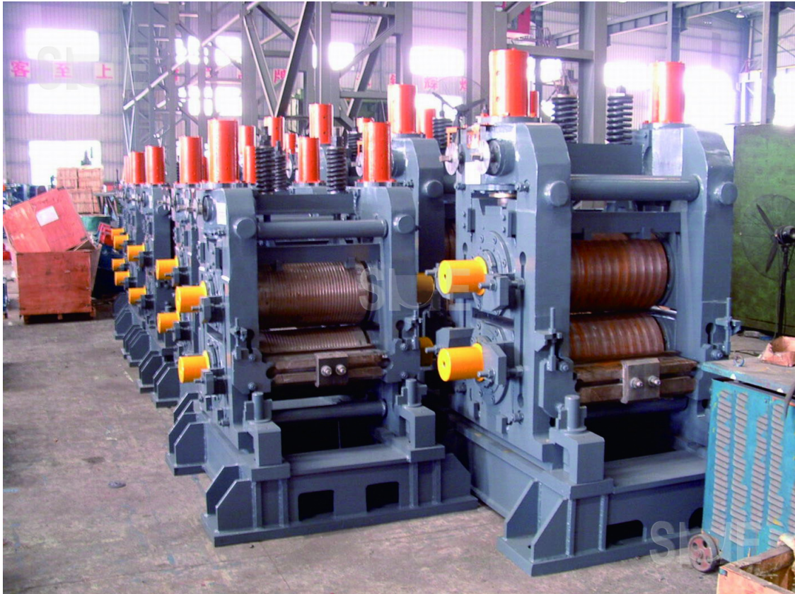
Figure 2.5: Hot rolling mill, made of several stands [18].
