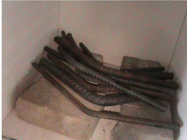
Figure 3.7: Bars packed in electric muffle furnace ready for ageing
