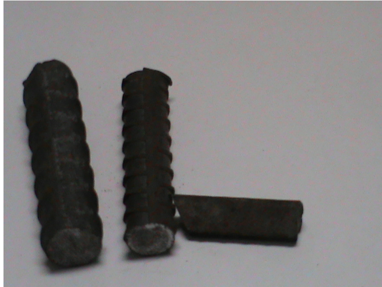
Figure 4.42: Bars end filed flat ready for chemical analysis, Source B
