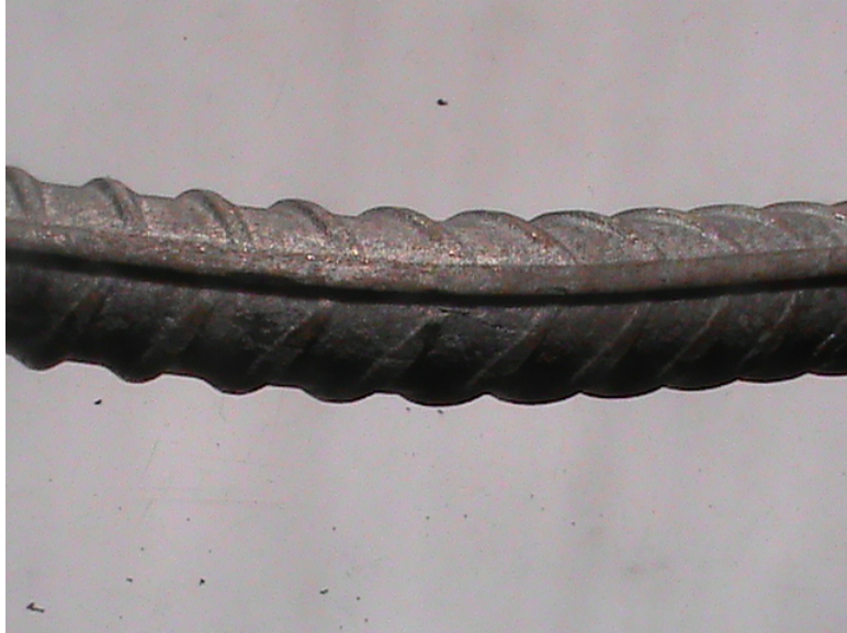
Figure 4.7: Visual of Rebar outside curve - source A
