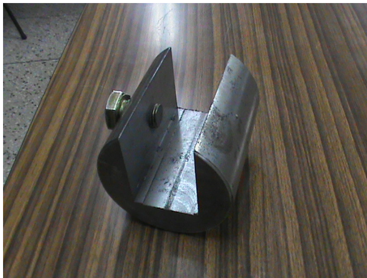
Figure 3.3: Milled modifier mandrel
