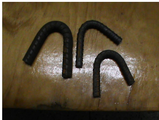
Figure 4.2: Bent rebars Source B
