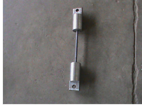
(b) Deformed bar mounted on grips and attached with epoxy steel
