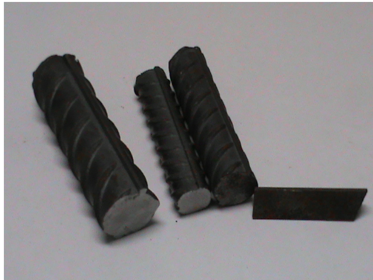
Figure 4.41: Bars end filed flat ready for chemical analysis, Source A
