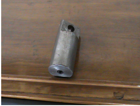
(a) The grip: notice axial hole for bar and lateral hole to interface with machine
