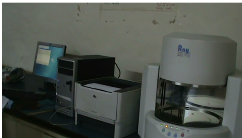
Figure 2.1: Energy Dispersive X-Ray (EDX) Spectrometer, (at PWD, Industrial Area)
