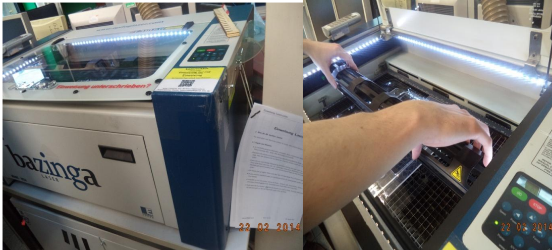
Figure 2.6: Photographs of a section of the CO 2 laser engraving/cutting machine (Epilog Helix 24) used to cut the cellophane segments at the technical science laboratory, University of Erlangen, Germany.
