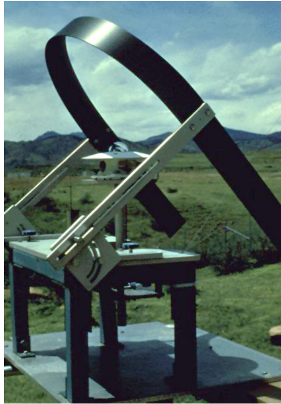
Figure 5 Shielded Pyranometer for diffuse solar radiation (WMO, 2008)
