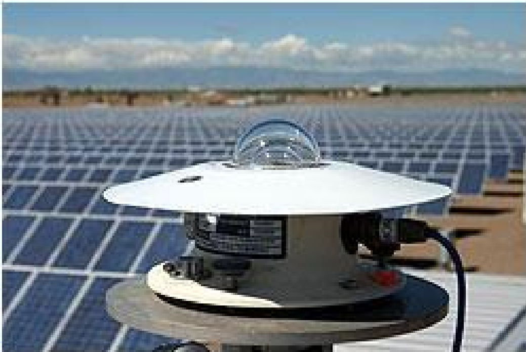
Figure 4 Unshielded pyranometer for global solar radiation (WMO, 2008).
