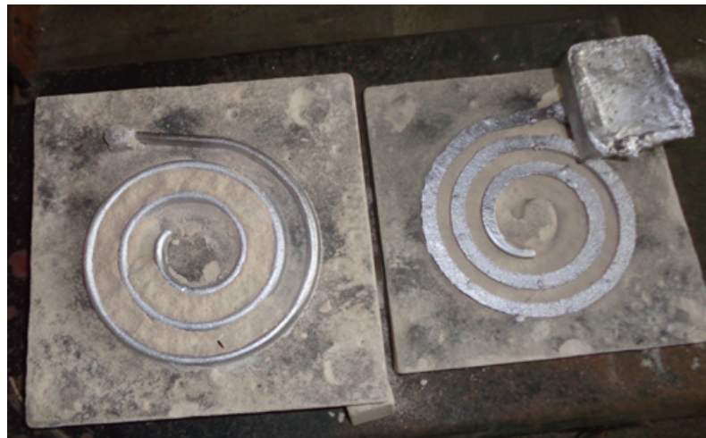
Figure 4.21: The outcome of the alloy's fluidity when it is solidified
