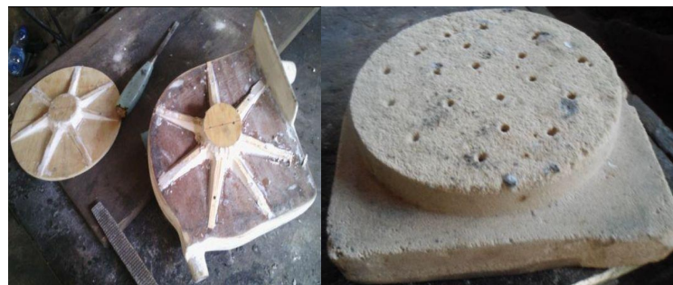
Figure A.6: Wooden pattern of the casing and sand core for the cavity of the turbine casing
