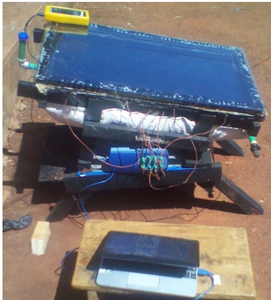
Plate 3.1: Typical experimental setup for the ICS cistern
