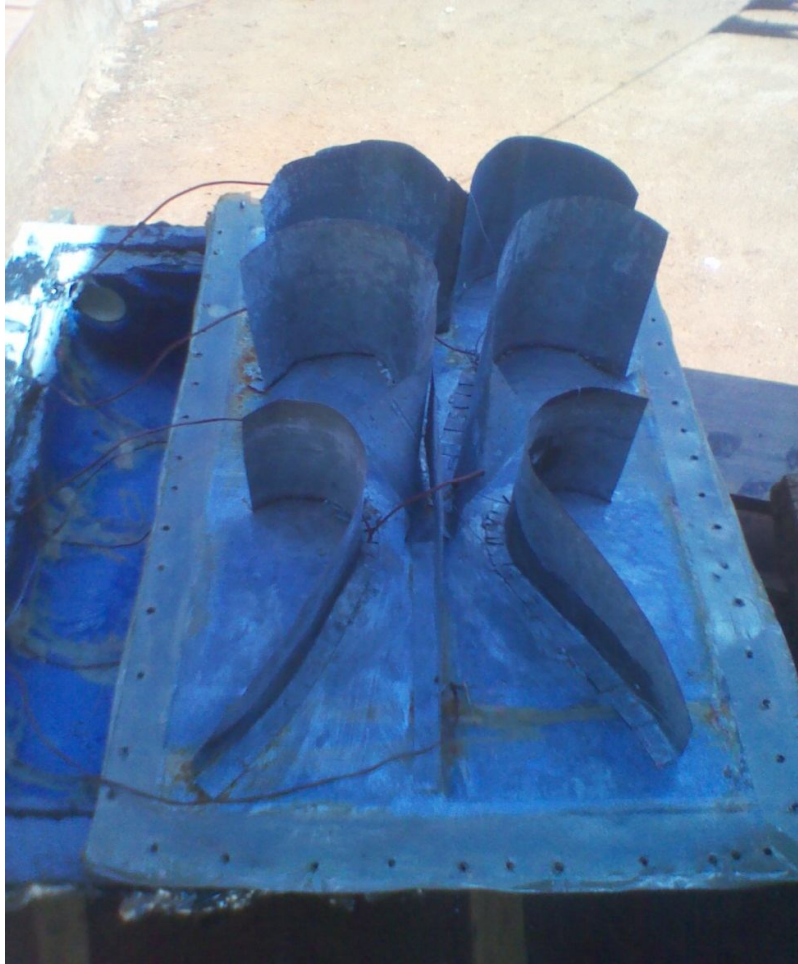
Plate C.4: Improved Absorber with a set of fins attached
