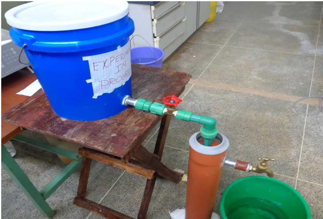
Plate 4.4: Photo of the Pilot Household Defluoridation Unit
