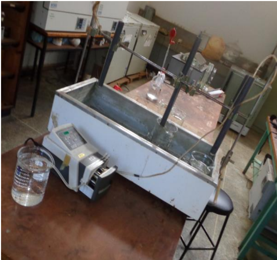
Plate 4.3: Experimental Photo of the mini column packed with crushed burnt clay pot
