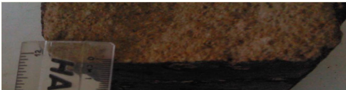
Plate 3. Degree of absorption of LDP melt on CSB Cured for 28 days
