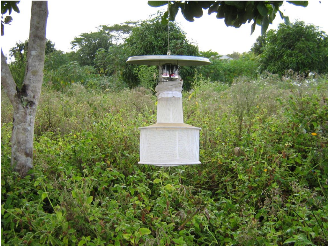
Plate 3:5 A CDC light trap hung outdoors on a cashew nut tree in Jaribuni, Kilifi
