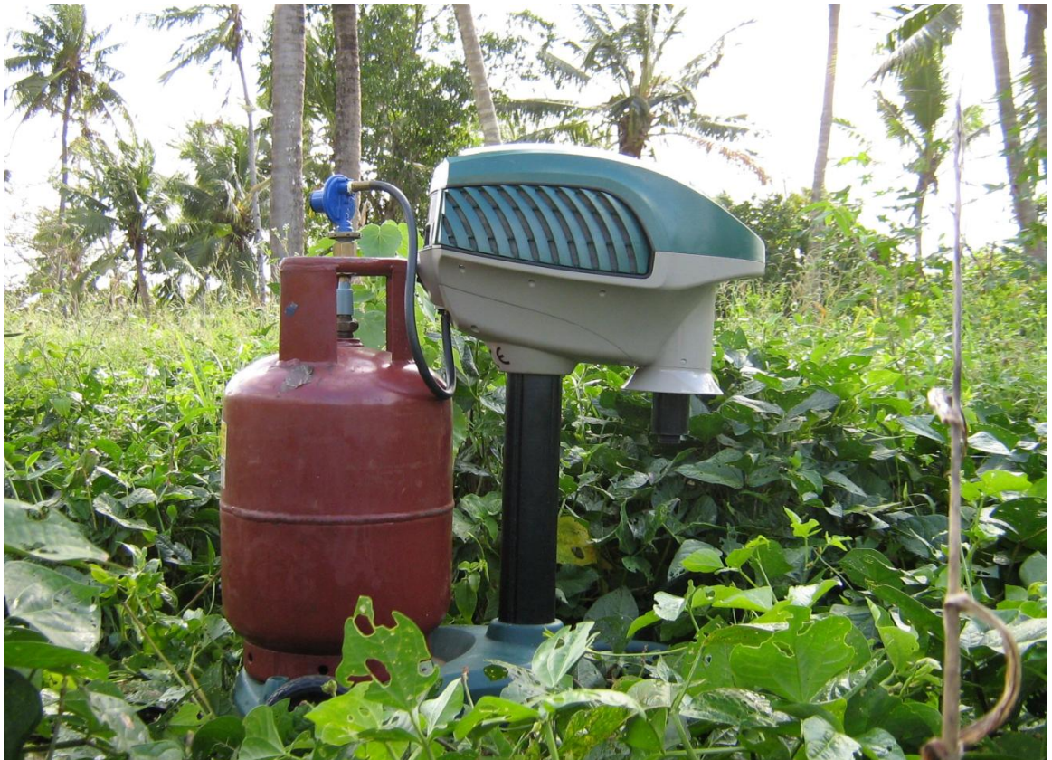
Plate 3:4 A mosquito magnet liberty plus trap set outdoors in a well vegetated area in Jaribuni, Kilifi.
