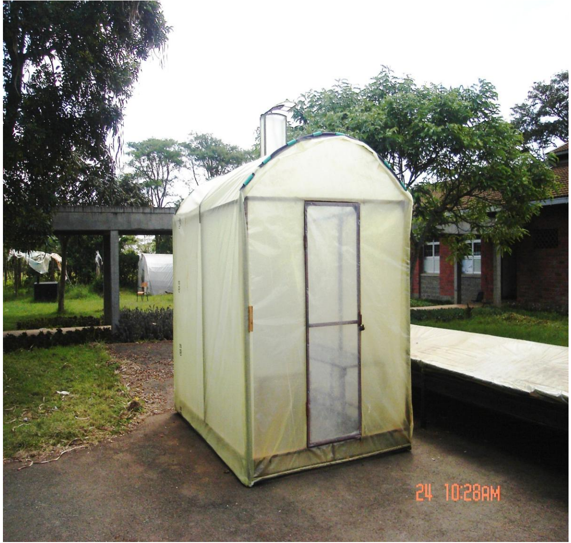
Plate C7 The actual solar tent dryer under natural convection.
