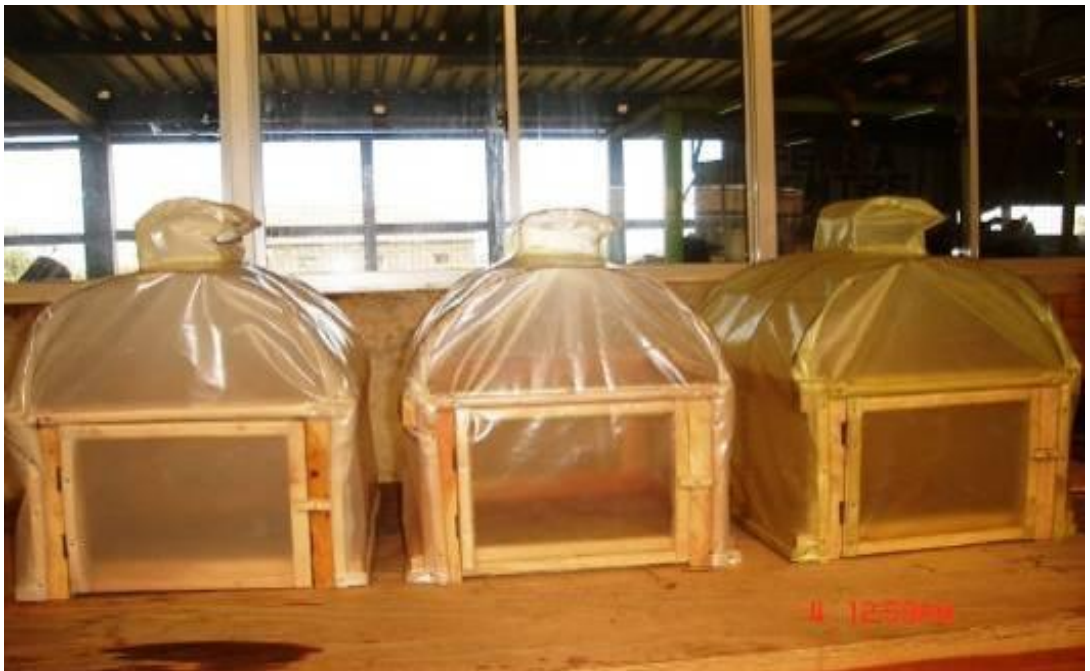
Plate C6 Developed model solar tent dryers with nectarine diffused, clear and yellow PVC cover materials.
