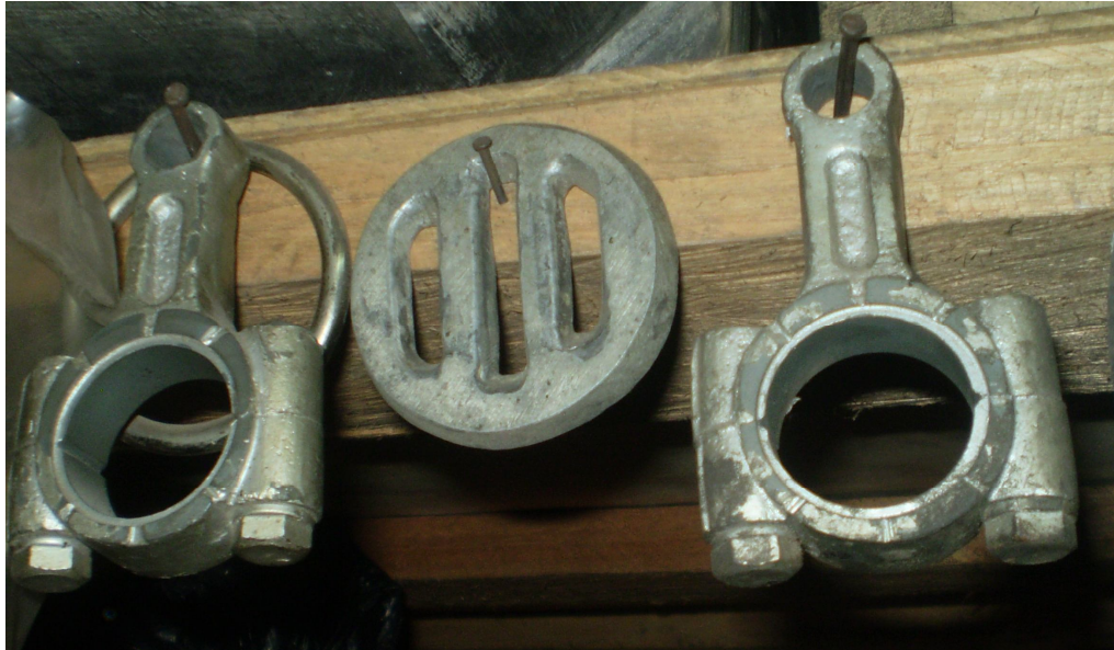
Figure 5.4: Automobile connecting rods with a strainer in between: Courtesy of Kariobangi Light Industries Ltd, Nairobi
