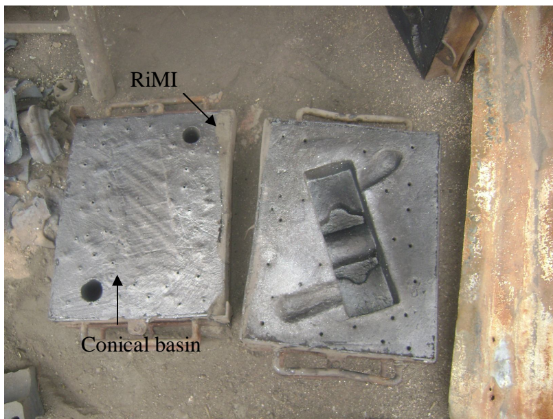
Figure 5.11: Sand mould with a conical basin for aluminium casting: Courtesy Hakika Engineering Workshop, Nakuru
