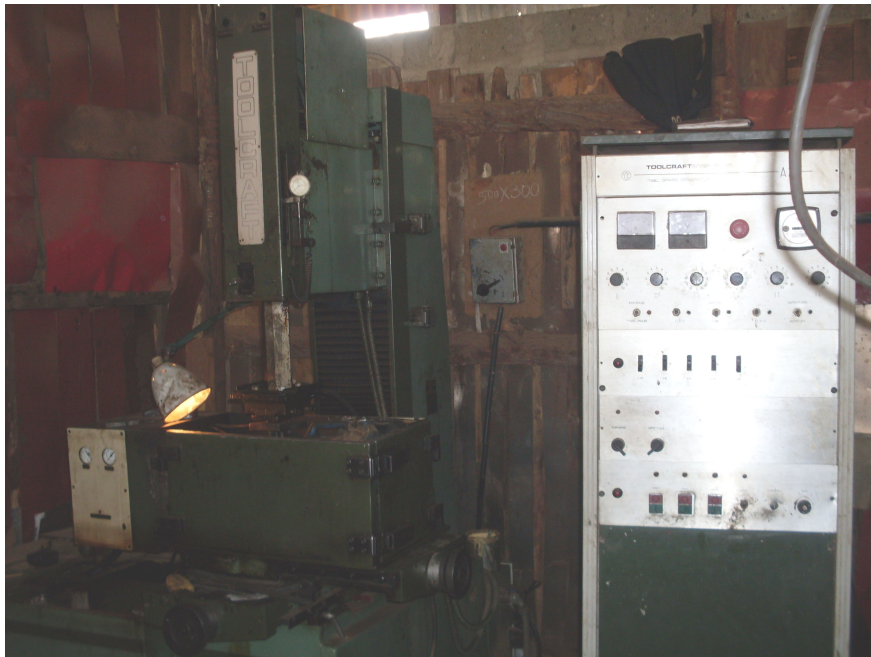
Figure 3.1: Electric discharge machine
