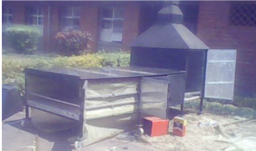
Plate A5: Solar tunnel dryer undergoing modification after optimisation
