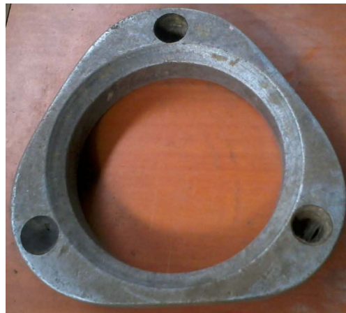
Figure 4.24: A motor vehicle spacer cast and finished in a kariobangi foundry
