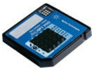
Figure 7: Agilent 7500 DNA chip used in library quality assay (GS FLX-Titanium System Technical Overview, Customer support- Genome sequencing- www.roche-applied-science.com )
