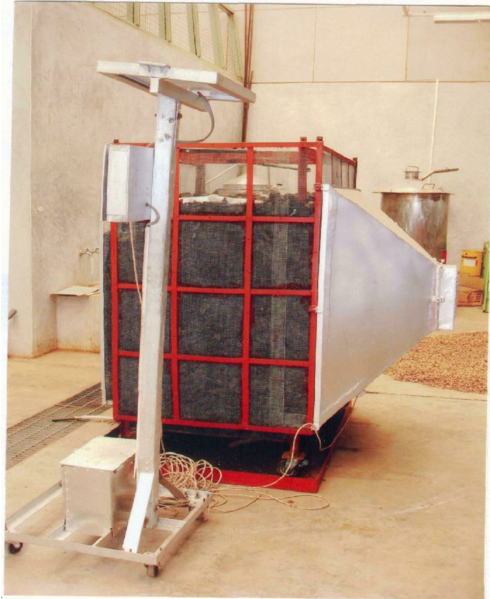
Figure 1: The prototype solar-charcoal cooler developed for laboratory studies
